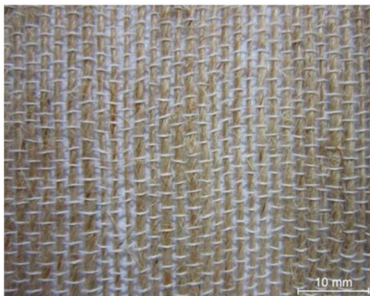
Figure 1. Structure of plain jute spun yarn fabric used in the present study.
